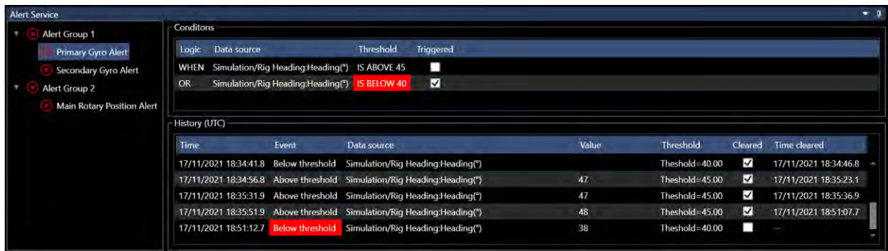
FIGURE 21-13 ALERT SERVICE VIEW WINDOW –CONDITION TRIGGERED
