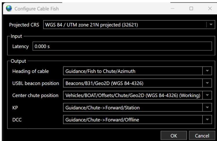
Figure 3 Cable Fish Output Configuration
