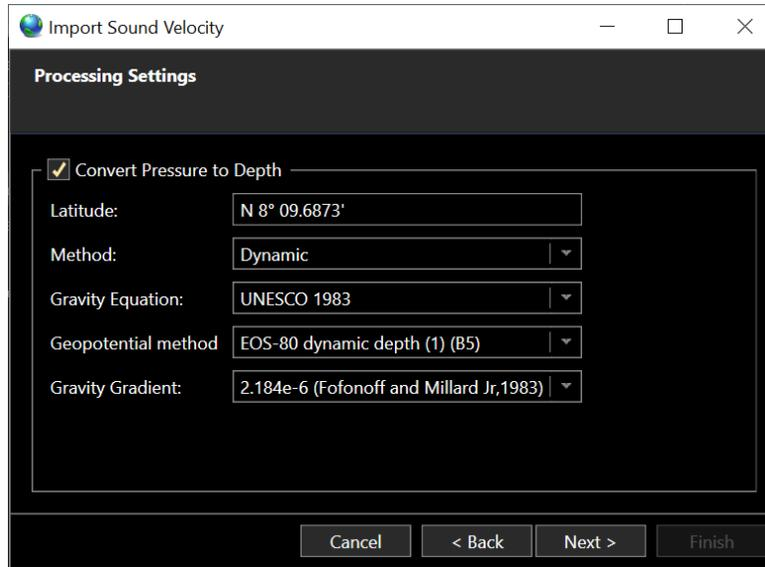
FIGURE 6 – IMPORT SOUND VELOCITY - PROCESSING SETTINGS
