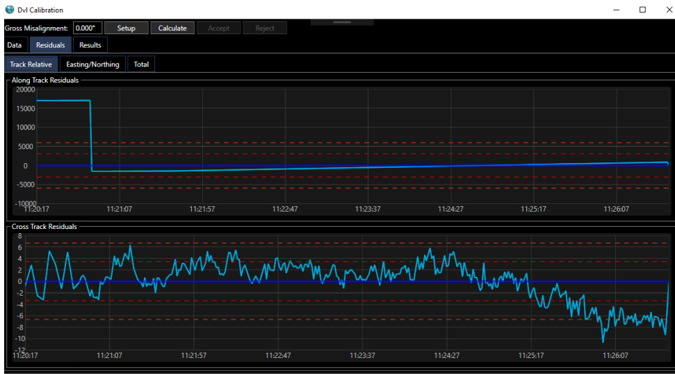
FIGURE 14-138 DVL CALIBRATION - HIGH RESIDUALS EXAMPLE
