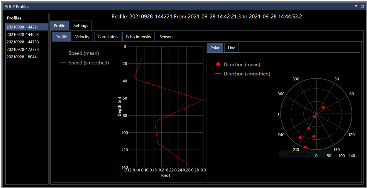
FIGURE 18-32 ADCP PROFILES - VIEW WINDOW
